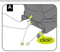
1. Pull the grey fabric loop (16) to pull out both locking arms (17) until you hear a clicking sound which indicates they are fully engaged.
