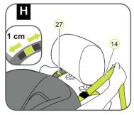
10. Tension the strap of the Top Tether (14) until the tension indicator (27) turns green and the Top Tether (14) is tightly tensioned.
