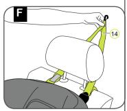
8. Guide the Top Tether (14) on the left and right-hand sides past the headrest
