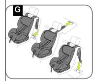
Hook the snap hook (26) into the Top Tether anchoring point recommended in your vehicle owner's auide
