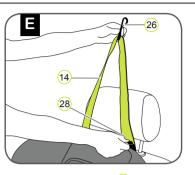
7. Take the Top Tether 14 and press the metal tongue (28) away from the strap to lengthen the strap and pull the Top Tether (14) by the snap hook (26) until it makes a V-shape.
