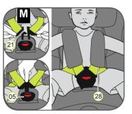
18. Guide the two buckle latches (21) together and engage them before putting them into the harness buckle 05 - this should make a clicking noise.
