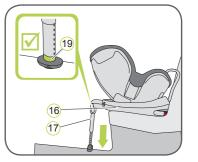
7. The support leg indicator (19) must be completly green
